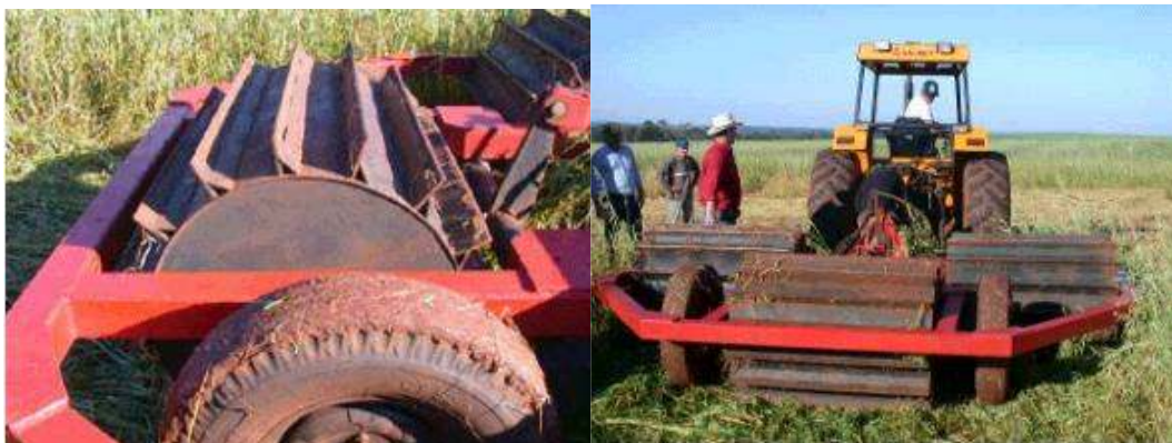
The knife roller was developed by farmers to flatten and break down cover crops before sowing
