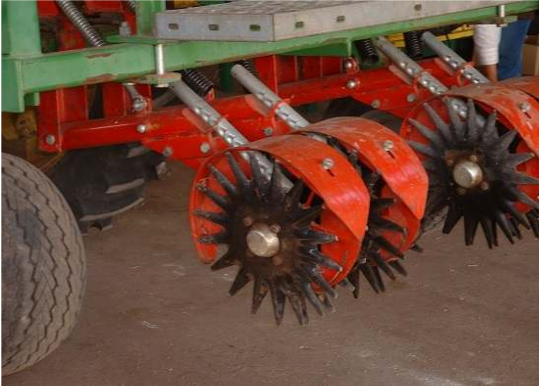
The star wheel seeding coulter can accurately place seed in soil by punching through crop residues
